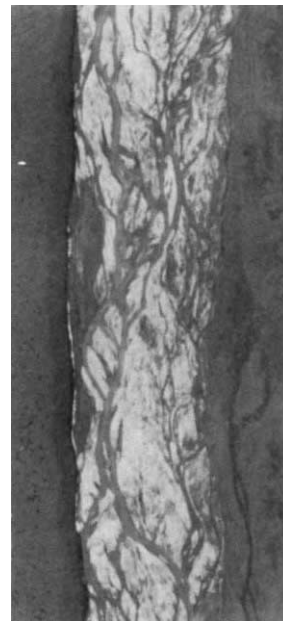
FIG. 1 Aerial photograph of part of the braided Aichilik River on the north slope of the Brooks Range in Alaska. Flow is from top to bottom. The slope is ~0.001, the gravel flat is ~0.5 km wide, and the flow depths are of the order of 1 m.
